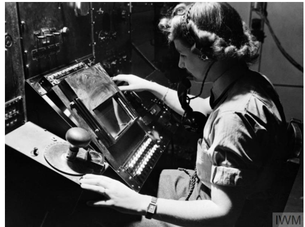
Fig. 1 WAAF radar operator Denise Miley plotting aircraft on the CRT (cathode ray tube) of an RF7 Receiver in the Receiver Room at Bawdsey CH 1 ,
